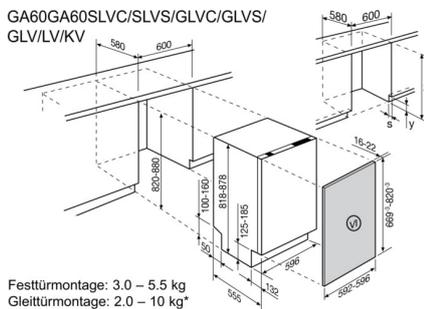
GA60SLVC/SLVS/GLVC/GLVS/GLV/LV/KV - eingebaut in
