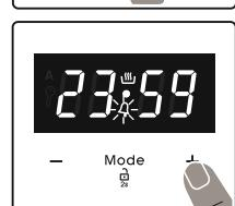
2. Select the desired time period using the "+" and "-" keys while "Q" is flashing.
